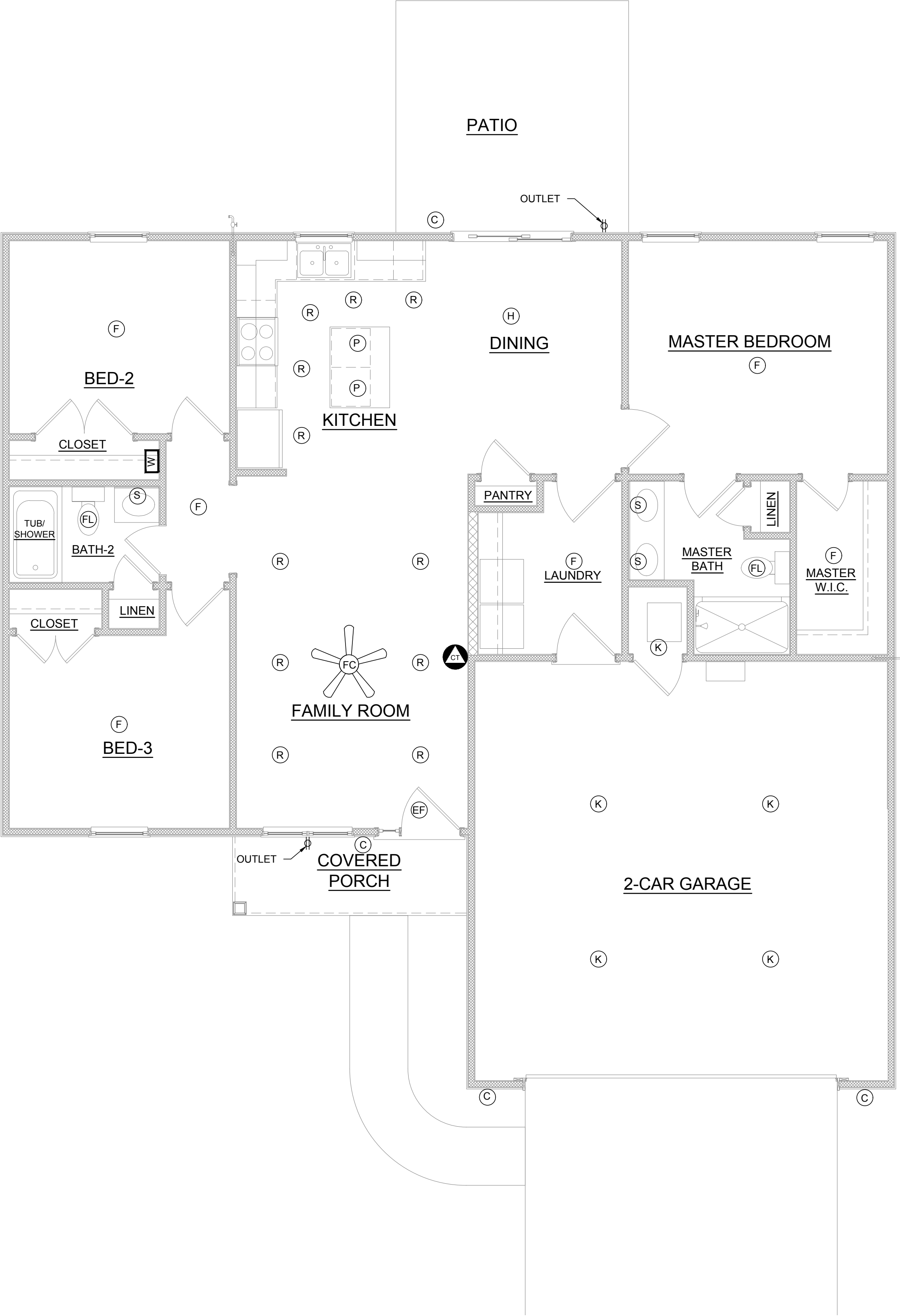
MAIN LEVEL ELECTRICAL PLAN SCALE: 1/4" = 1'-0"
